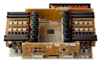
Glass cloth fluorocarbon resin PC-board
