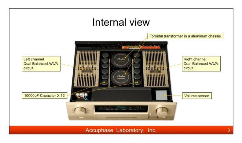
C-3900 inherits C-3800's internal construction as it is.
