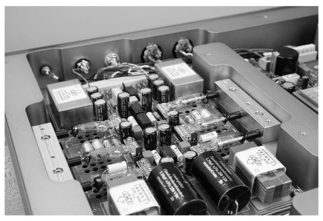
All tube amplification with six pieces of sub miniature vacuum tube
