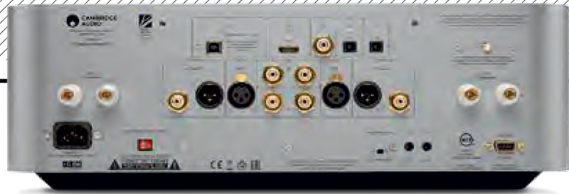
ABOVE: Two line ins (on RCA and balanced on XLR) are joined by variable pre outs (RCA and XLR) plus digital ins on optical (x2), coaxial, HDMI (audio return channel), USB-B (384kHz/32-bit, DSD256) and wireless (Bluetooth aptX HD)
